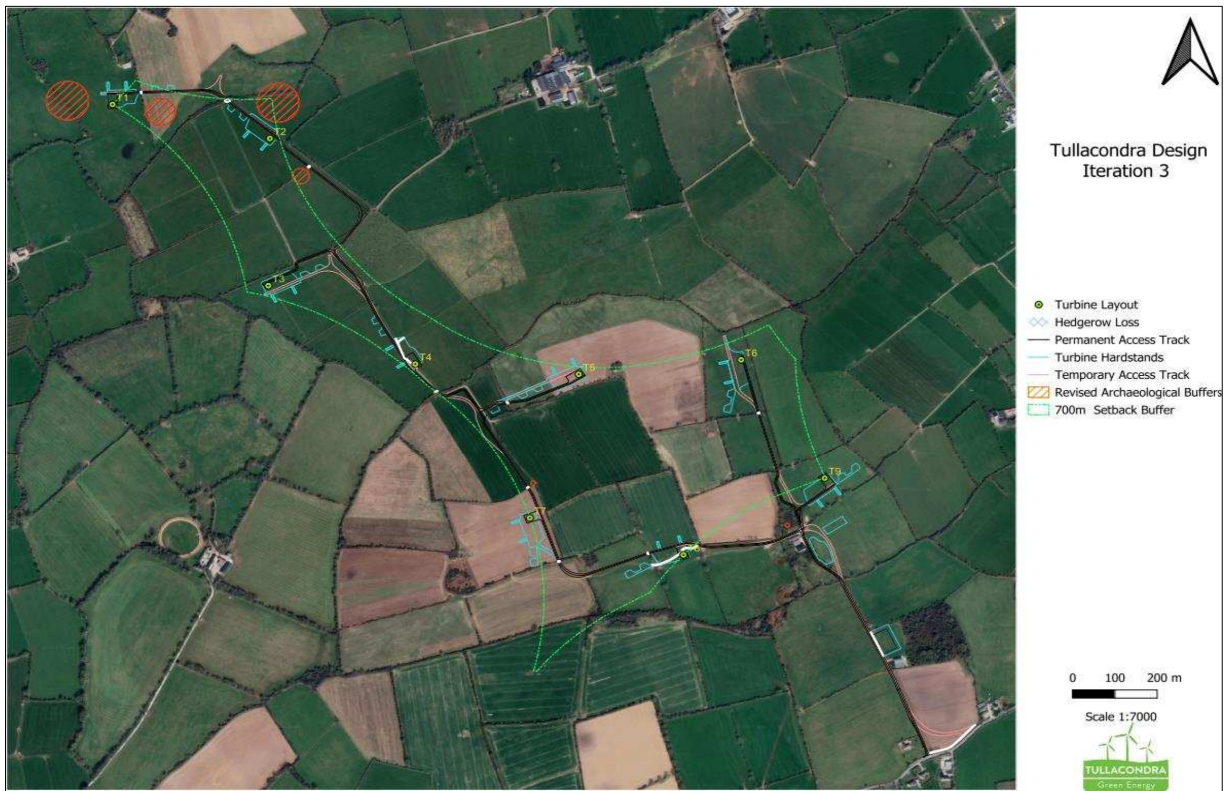
Figure 4.9: Final layout (Design Iteration 3) with minimal hedgerow loss
