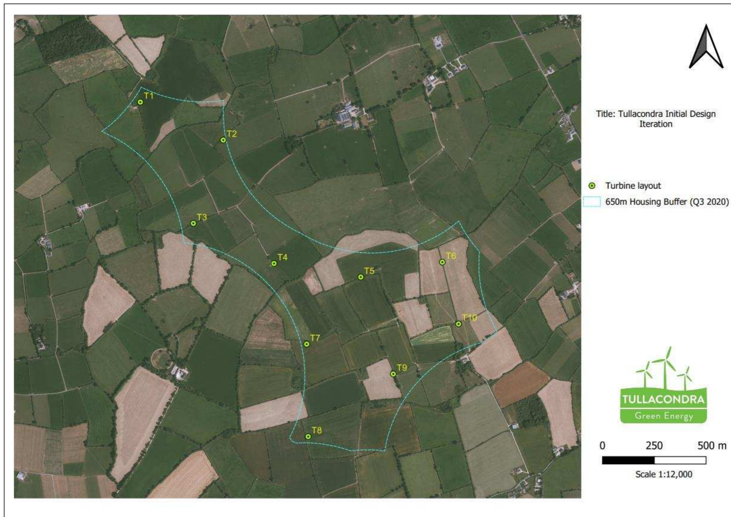
Figure 4.4: Initial 10-turbine layout
